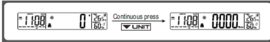
Note: if you press the "Unit" button shortly, you will switch to water/milk volume measuring mode (see below). A continuous press on the "Unit" button is requested to switch between measurement systems. The system by default is imperial.
